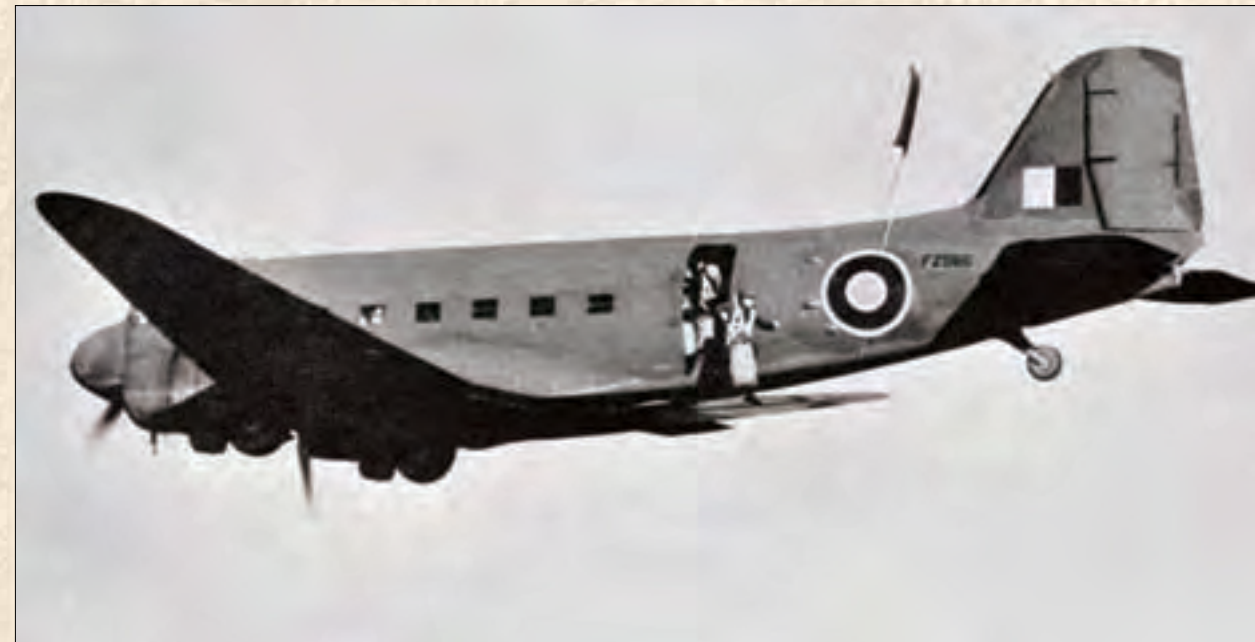
Above: Jumping from a Dakota. The static line pulls the parachute from the pack after exiting the aircraft. Standing tightly together, up to 20 men could jump in this way at the rate of about one a second. The plane is travelling at 200 feet a second and any slow jumping will result in wide separation of the parachutists when they land. Note the kitbag on the man's leg.
