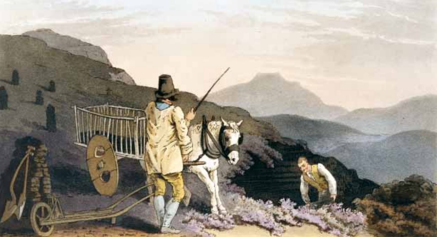
▲ A peat cart in Langstrothdale, source of the uppermost reaches of the river Wharfe. The thin wheels enabled the cart to pass easily through turf. The author of The Costume of Yorkshire observed that in 1814 peat was the general fuel used in the mountainous and moorland districts of northern England, and that it was customarily dug or cut into pieces about the size of a common brick, before being dried by the sun and stacked before use. Hand-coloured aquatint by Robert Havell after George Walker.
